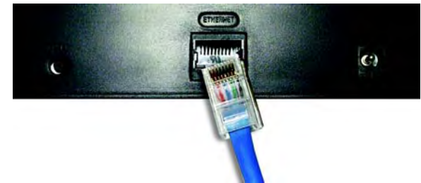
Figure 4-1: Connect the Ethernet Cable
