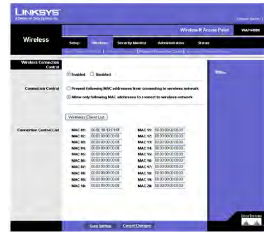
Figure 6-14: Wireless - Wireless Connection Control
